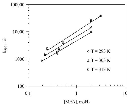
**Figure 8.** Experimental results of the apparent reaction-rate constants for CO<sub>2</sub> reaction with aqueous MEA solutions.
