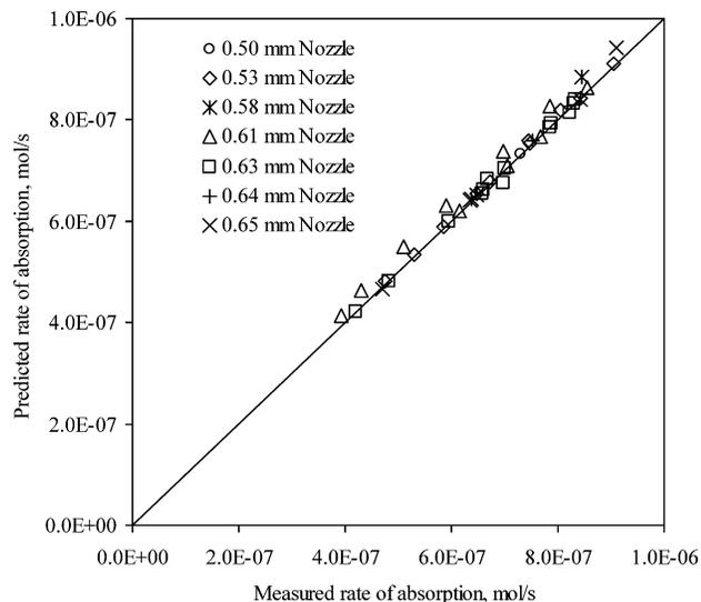
**Figure 5.** Comparison of measured and predicted CO<sub>2</sub> absorption rate into water at 298 K in the laminar liquid jet absorber.
