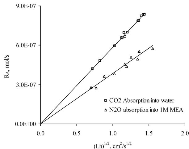
**Figure 4.** Physical absorption rates of CO<sub>2</sub> into water and N<sub>2</sub>O into 1 M MEA solution at 298 K and atmospheric pressure in laminar jet absorber: experimental (points), and theoretical (line).
