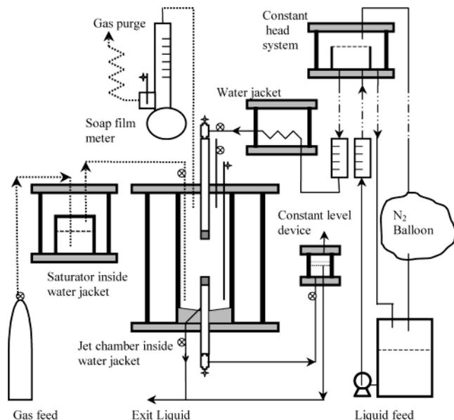
**Figure 1.** Schematic drawing of the laminar jet apparatus.
