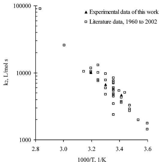
**Figure 9.** Arrhenius plot for the reaction between CO<sub>2</sub> and aqueous MEA solutions.
