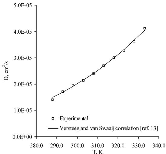
**Figure 6.** Diffusivity of CO<sub>2</sub> in water as a function of temperature.
